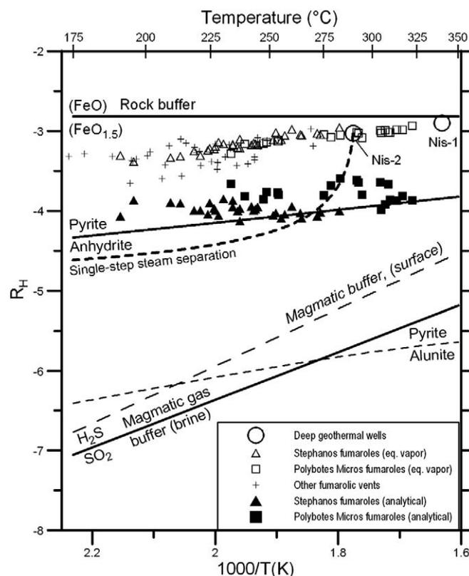
**Fig. 5.** Values of  $R_H$  as a function of temperature for the liquid phases tapped by the deep geothermal wells Nisyros-1 and Nisyros-2 as well as those feeding the fumarolic vents of the hydrothermal craters' area. Also shown are both different redox buffers acting in hydrothermal–magmatic environments and the effects of single-step steam separation on the Nisyros-2 liquid phase (from Giggenbach, 1987, modified).
