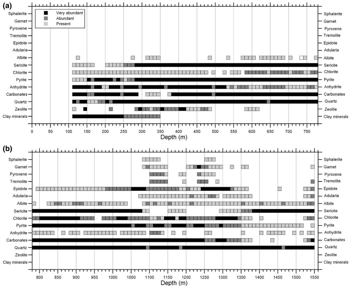
**Fig. 4.** Log of hydrothermal mineralogy in well Nisyros-2. Low-temperature minerals (clay minerals and low-temperature zeolites) are positioned in the bottom lines. Above are the ubiquitous solid phases, namely quartz, carbonates, anhydrite, pyrite, chlorite and sericite. In the top lines are found the high-temperature minerals, namely albite, adularia, epidote, tremolite, pyroxene, garnet and sphalerite (from *Geotermica Italiana*, 1984).
